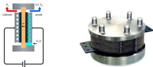
Figure 44: PEM cell schematic 1 (left) and real 1 kW PEM stack 2 (right)
