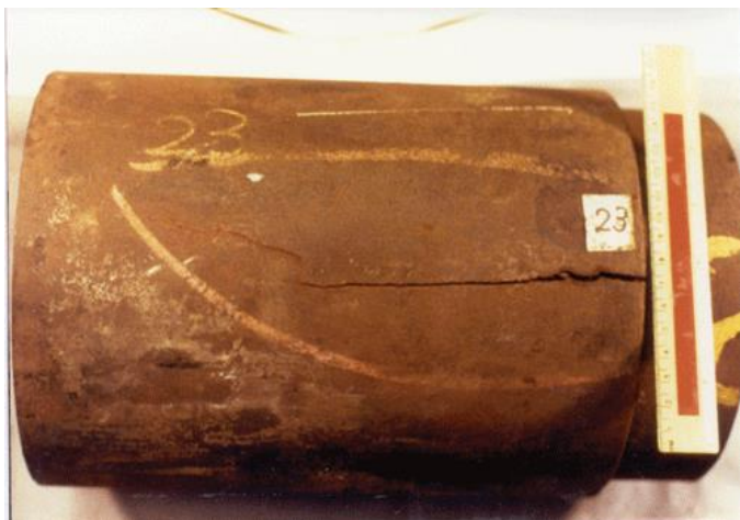
Figure 113: Metal cracking resulting from hydrogen embrittlement 4
