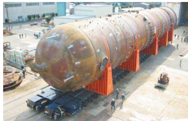
Figure 149: SASOL-Chevron Fischer-Tropsch reactor
