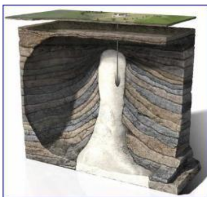
Figure 69: Illustration of a salt cavern 1
